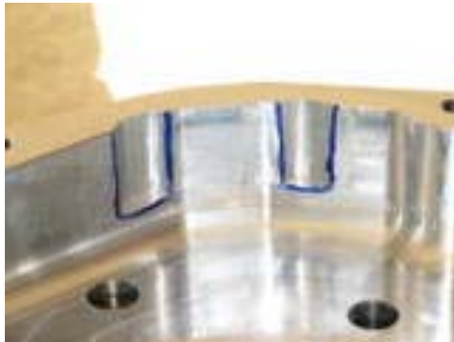
Rear tail housing cleared to clear shift rails.
