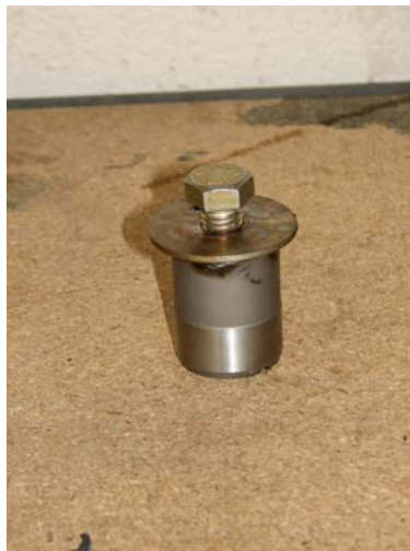
Stock transfer case coupler removed with large bolt and nut tack welded in place.
