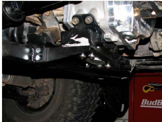
Additional transfer case mount and bracket.
