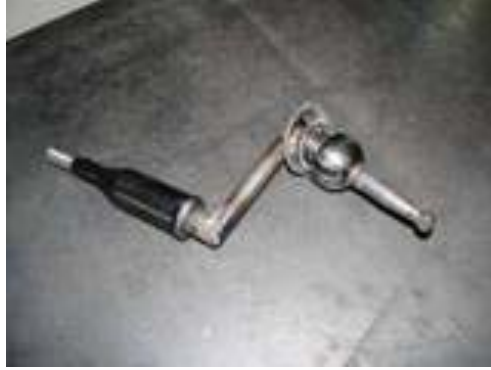
"Doglegged" TC shifter with short shift mod.
