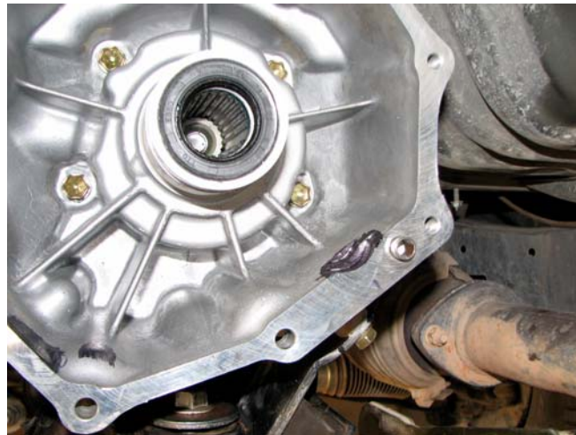
Coupler installed, Marlin oil seal housing and seal, tail housing notched and re-installed
