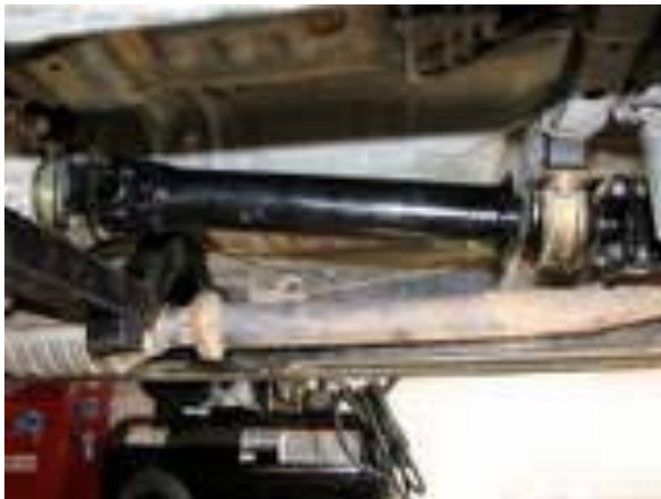
Front section of rear driveshaft shortened 8.5"
