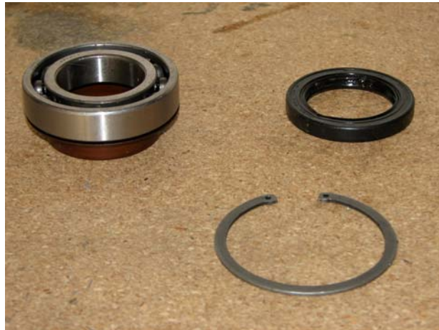
Stock tail housing bearing, oil slinger, seal, and circlip removed.
