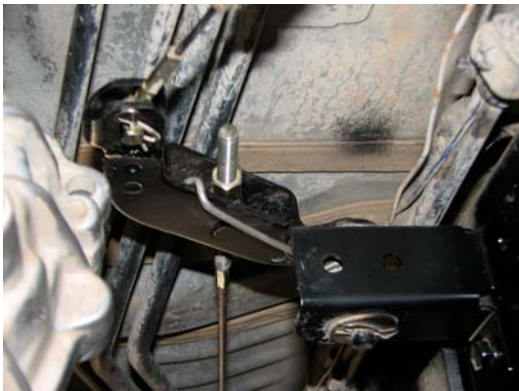
Parking brake bell crank assembly modified
