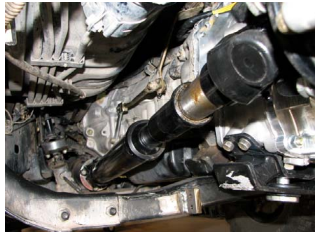
Front driveshaft lengthened 8.5"
